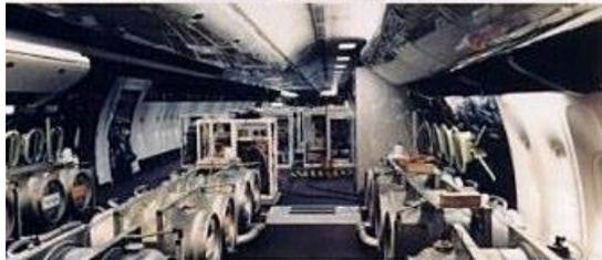
During flight tests in 1994, the cabin interior of the prototype 777 was filled with what at first glance looked like aluminum beer kegs. In fact, these 55-gallon barrels contained water. The contents of two dozen barrels in the forward cabin and a like number of barrels in the aft section were pumped back and forth to simulate shifts in center of gravity that would result from passengers moving about. The top photo shows the cabin as it is when the 777 is delivered.
