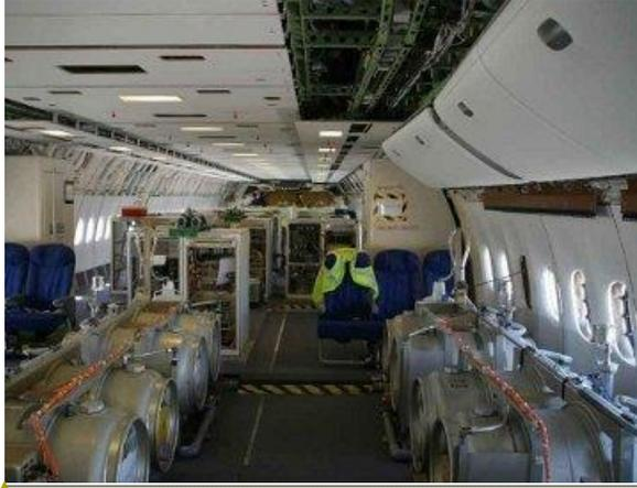
What are the barrels for? Do they contain barium or other heavy metals? According to the below page of a Boeing manual, these barrels were used in a test. The barrels contained water and were used to simulate the movement of fluids in human passengers.
